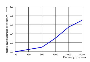
Weighted sound absorption coefficient according to ISO 11654
